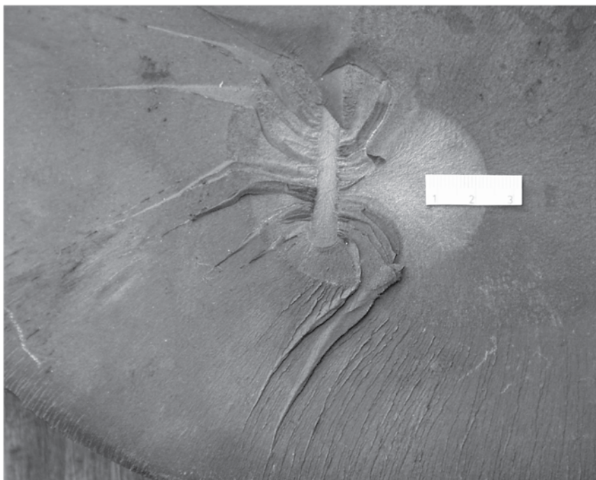
Fig. 1: Spalling fracture of the roll
